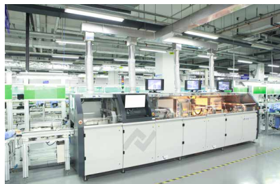
Automatic Welding System
