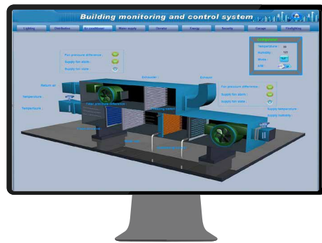
HMI for Building Management
