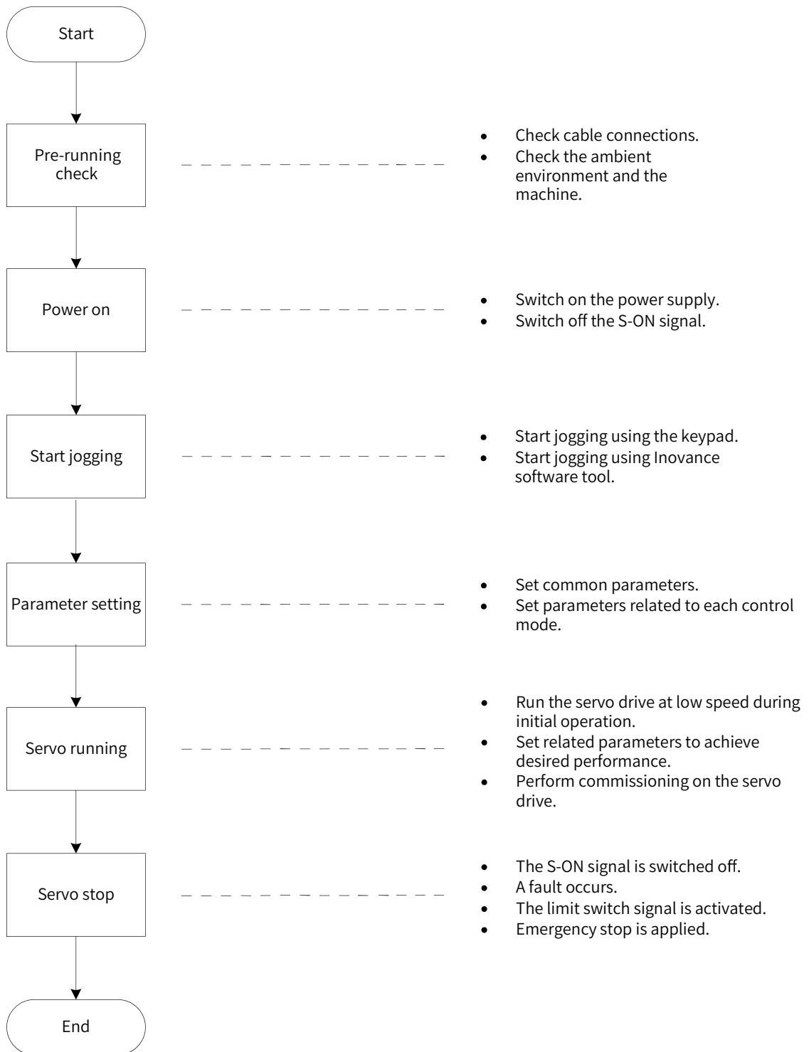
Figure 5-1 Flowchart for setting the servo drive
