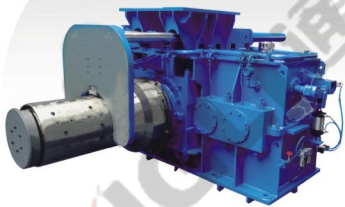
| 精轧卷取机用减速机 Precision Uncoiler Specialized Gearbox
