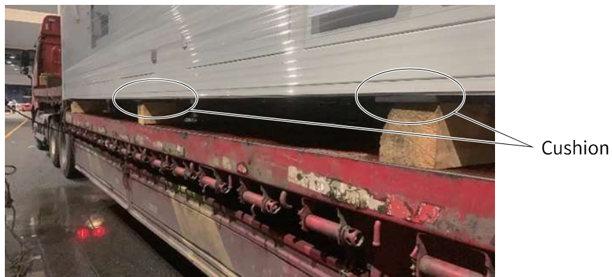
Figure 3-8 Rubber cushion under the equipment
